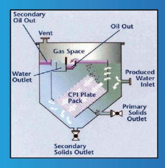
CPI Separators enhance oil-water separation through corrugated plates that increase the surface area for coalescing oil droplets, providing efficient removal of oil and suspended solids from wastewater.
