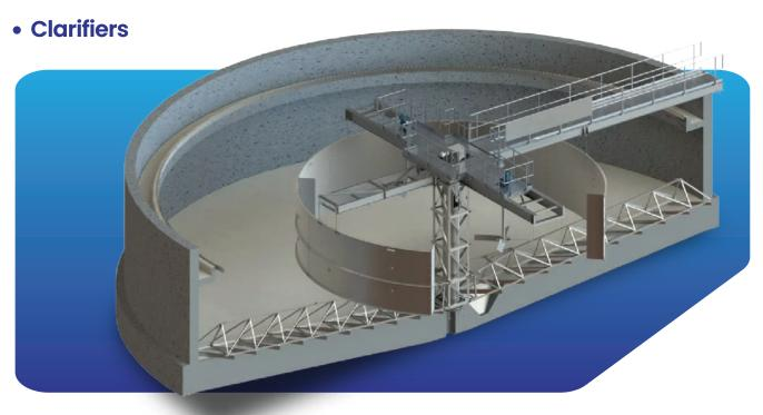
Clarifiers are used to settle suspended solids from wastewater, producing clear effluent and concentrated sludge. These systems are fundamental in primary and secondary wastewater treatment processes.
